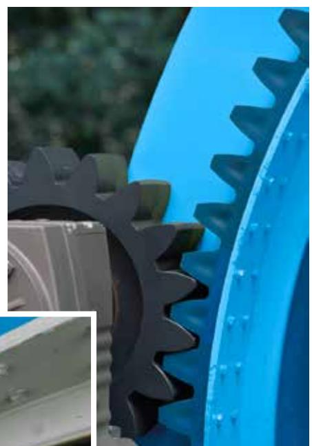
**The TSA is driven by a patented gear sprocket with individually exchangeable segments.**
