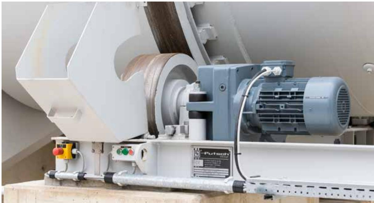
**The drum is supported by four support rollers which are operated by gear motors.**
