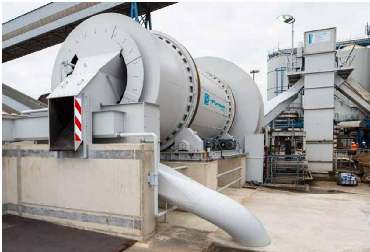
**Putsch® SAT stone preparation drum (foreground) directly supplied by the Putsch® GSA belt stone separator (background).**
