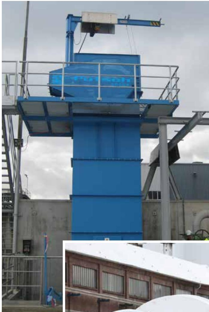
**The work platform on the top section of the GSA enables maintenance work on the drive and bucket elevator. The lifting device for buckets over the top section additionally eases the operator's work.**
