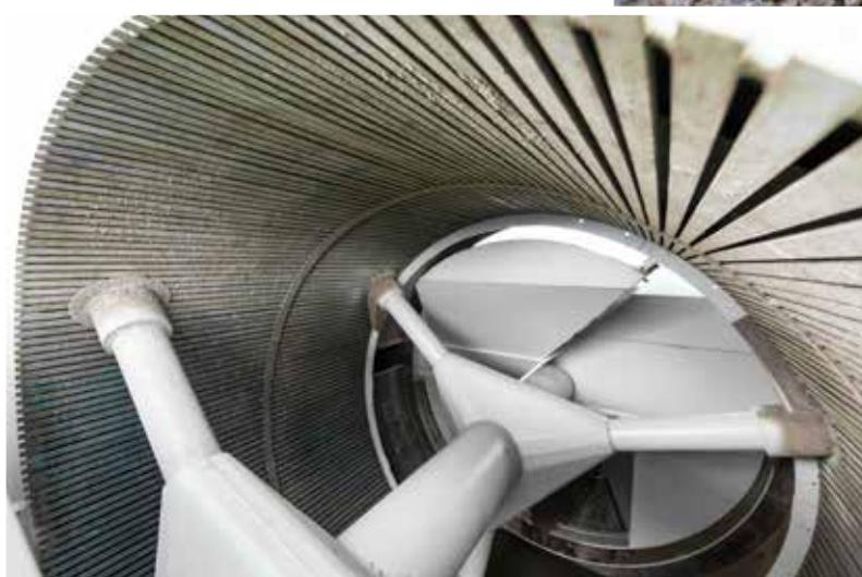
**Putsch® TSA are equipped with a self-cleaning screen drum.**
