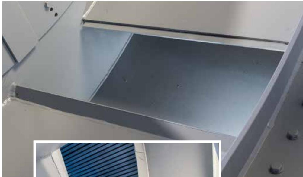
**Adjustable stone pocket covers change the cross-section of the stone pocket openings and thus regulate the speed of the buoyancy water.**
