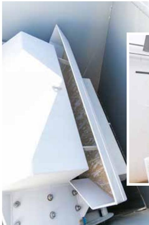
**Scraper buckets continuously remove the sand and gravel deposits from the base and transport it away with the stones.**
