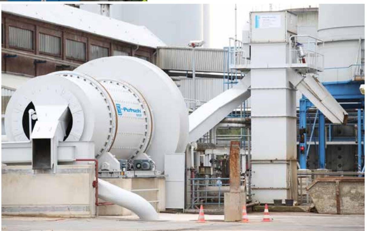
**The optional second discharge chute transports the stones directly into the Putsch® stone preparation drum or the stone box.**
