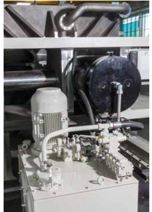
Low costs due to a simplified hydraulic system and shorter hydraulic cylinders.
