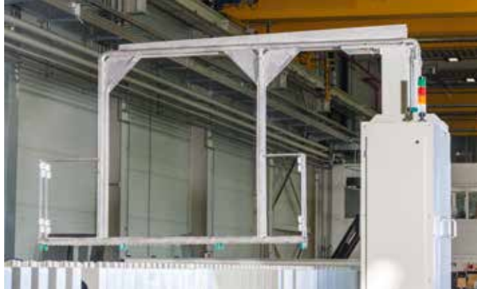
An automatic washing machine cleans the filter cloths quickly and efficiently.
